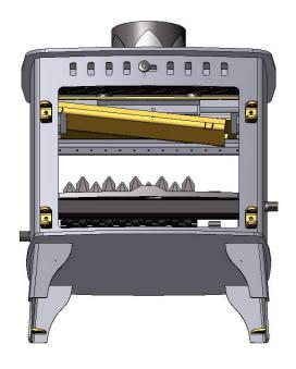
Remove the Location Pins from Turbo Bar. Slide it to the left. Once clear of the R.H. Turbo Duct pull it towards you and out of the L.H. Turbo Duct.
