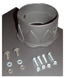
Place the Flue Gasket on the Top Plate Flue Exit. Place the Flue Collar on top of the Gasket. Secure to the four locating tabs, inside the flue outlet, using the M6 nuts & bolts supplied. Fit the 2 - M8 carriage bolts, washers & nuts into the Damper Holes, located on each side of the Flue Collar.
