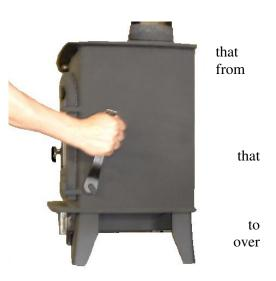
The ashpan should be emptied at least daily and ash should never be allowed to build up over a period of time as this will result in damage to the fire bars. The flat end of the riddling tool can be used to carry the ashpan.
