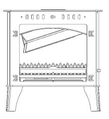
Lift the Baffle and slide to the right. When the left side of the baffle clears the support, lower the baffle into the Fire Box and remove. Refit in reverse order making sure that the back edge of the baffle is located between the two baffle supports.
