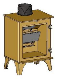
Pull the top edge of the Rear Brick towards you, lift and remove.
