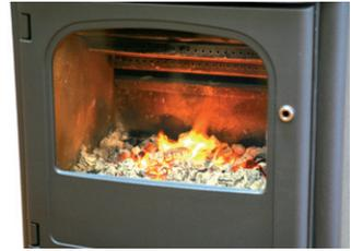
6. Place three pieces of fuel weighing roughly 0.6 kg and measuring about 25 cm in length across the embers in one layer, with spacing of roughly 1 cm between the pieces of wood.
