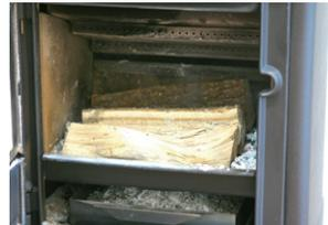
8. Once the new fuel has taken, adjust the secondary air amount to the desired setting; optimal combustion will continue until glowing charcoals are produced. Under normal chimney draft conditions, expect to re-fuel your stove every 60 - 70 minutes.
