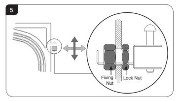
Use a 19mm A/F spanner to loosen the fixing nuts.
