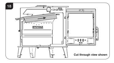
3b.3 Move the baffle to the right, lift the left side and slide on to the support pin, see Diagram 19.
