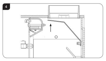
4.7 Rotate the baffle forwards over the top of the support pins, see Diagram 5.
