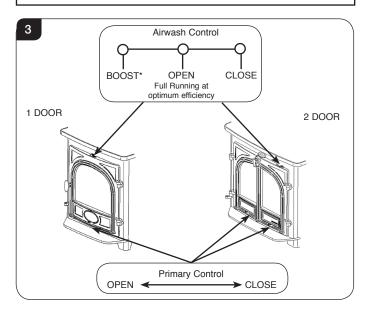
\* The **boost setting** allows for quicker start up and glass cleaning only. DO NOT run the appliance on this setting for extended periods of time.
