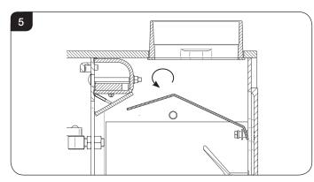
4.8 Lift the rear of the baffle to disengage from the bolts at the back of the stove and continue to rotate, see Diagram 6.
