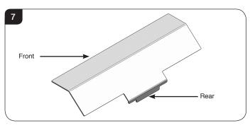
Ensure that rear of the baffle engages between the bolts at the back of the appliance, see Diagram 8.
