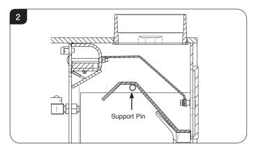
4.5 Rotate the baffle to remove from the firebox through the door opening.
