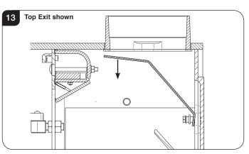
Ensure the front of the baffle is positioned on top of the front bolts and rests against the front of the firebox, see Diagram 14.
