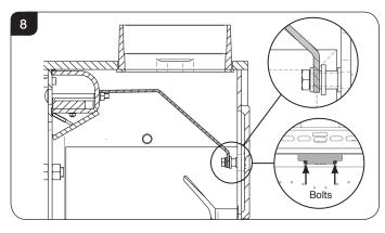
4.10 Ensure the front of the baffle is positioned on top of the front bolts and rests against the front of the firebox, see Diagram 9.
