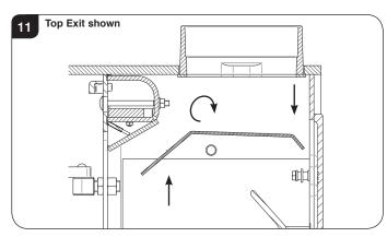
2.3 Rotate and lower the rear of the baffle, ensuring that it engages between the bolts at the back of the appliance, see Diagram 12.
