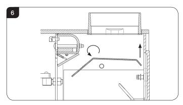
4.9 Continue to rotate and lower out through the door opening.
